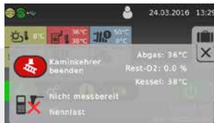
Fig. 2 View of the chimney sweeper function
